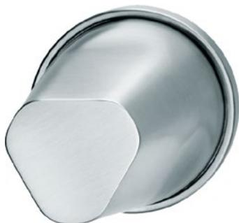
Door knob of particularly rugged construction in the shape of a stub-ended cone with gripping recesses, its shank enclosed within a special-purpose rose. It is impossible to attach cords or ropes to the knob. Its ergonomic form guarantees good gripping qualities and lessens the likelihood of acts of suicide.
