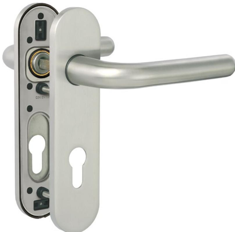
Lever set with short, invisibly fixed backplates, equipped on the female-handle face with fixed lugs. This “female” hardware is fitted on the inside of the room so as to prevent its being tampered with or dismantled. The levers are rotatably fixed on either side and are designed to cope with heavy use. The screw fixings on the outside face are concealed by an outer backplate that is securely clipped fast.
